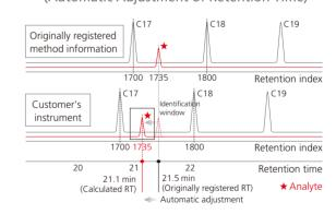
The AART function adjusts the retention times of target components based on linear retention indices (LRI) and the retention times of n-alkanes. The AART function easily adjusts acquisition and processing method parameters simultaneously.
