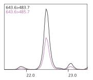
Example of PBDE Analysis in Sediment Column: Rtx-1614 (30 m, 0.25 mm, and 0.1 mm) 2,2', 4,4', 5,6'-Hexabromodiphenyl ether (#154) (0.436 ng/g concentration in sediment)
