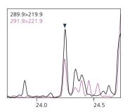
Example of PCB Analysis in River Water Column: Rtx-PCB (60 m, 0.25 mm, and 0.25 mm) 2,2', 5,5'-Tetrachlorobiphenyl (#52) (0.080 ng/L concentration in water)
